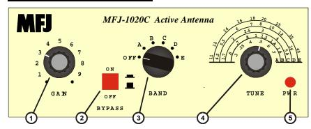
1. GAIN CONTROL:.....Adjust the gain of the MFJ-1020C from -10 dB to +10 dB.
